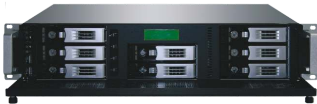
NDL-2800SR with closed and open door for 8x SAS/SATA HDDs
