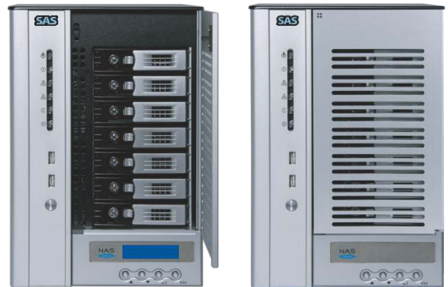
NDL-2700ST with open and closed door for 7x SAS/SATA II HDDs
