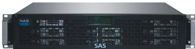
NDL-2800SR with closed and open door for 8x SAS/SATA HDDs
